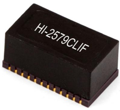
Holt Integrated Circuits today announced the introduction of HI-2579, the World's smallest 3.3V MIL-STD-1553/1760 dual transceiver with integrated dual transformers.
