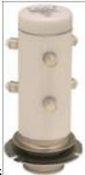
GIGAVAC has introduced a new DPDT 20kV relay. The G53WF is ideal for applications requiring high continuous carry current, up to 150A, as well as high power RF circuits that require low signal loss. The combination of massive copper contacts and a vacuum dielectric provide a low and stable 12 milliohm contact resistance which means low voltage drop in DC circuits and low signal loss in RF circuits.
