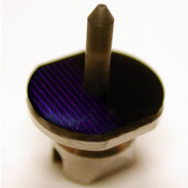
Count On Tools announces a breakthrough in custom nozzle engineering for ultra-smooth components from the semiconductor market. The latest series of nozzles feature precision-machined urethane tips that prevent components with very fine surface finishes, such as bare dies and wafer level components, from getting stuck on the nozzle tip during the pick-and-place process.
