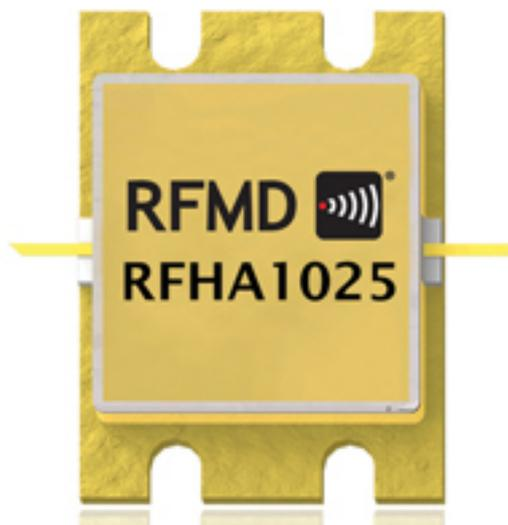
RF Micro Devices today announced the release of the RFHA1025, a highly-efficient 280-watt pulsed gallium nitride (GaN) RF matched power transistor. The RFHA1025 delivers superior performance versus competing silicon power technologies.
