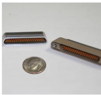
SOURIAU PA&E's new Mini-Micro-D connectors are designed for space, airborne, down-hole oil and any other hermetic applications where reducing size and weight are priorities. They have a 27% lower profile than standard Micro-D connectors and are designed to be laser welded into aluminum, titanium or kovar housings. These new hermetic connectors are MIL-PRF-83513/7 interface compliant and mate with connectors manufactured to MIL-PRF-83513/8.
