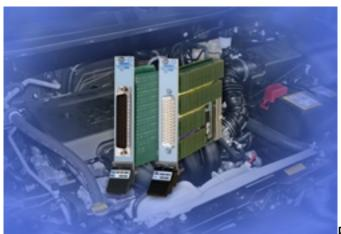
Pickering Interfaces is expanding its range of PXI Fault Insertion solutions with the introduction of the 40-197 and the 40-198. Fault Insertion (FI) modules are used within an Automatic Test System to simulate common fault conditions such as an open, short to ground or a short to other connections in a device under test.
