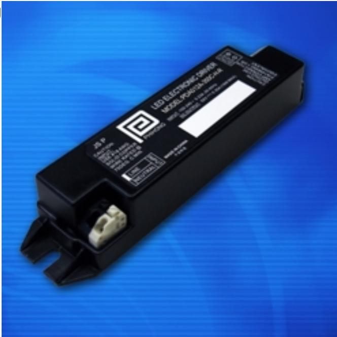
, a global leader in power and energy-efficient lighting solutions, has developed a series of 12W drivers for indoor LED lighting. Designated the PDA012A (for AC input of 220-277VAC) and PDA012B (for AC input of 100-120VAC), the 350mA constant-current driver operates at an output voltage range of 10~43VDC and is ideal for applications such as display lighting and strings of a few high-intensity bulbs.
