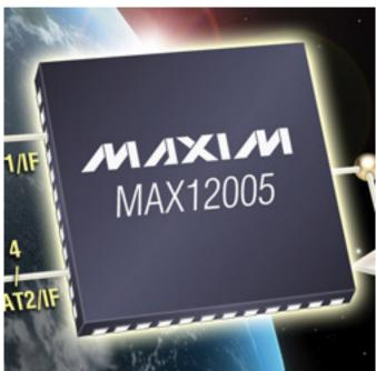
Maxim Integrated Products introduces the MAX12005, the industry's first 8 x 4 satellite IF switch IC that is expandable to allow up to 16 satellite signals. Highly integrated, the MAX12005 is flexible and adaptable for a wide range of space-constrained, satellite IF distribution and multiswitch applications.
