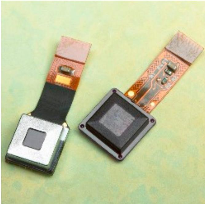
Avago Technologies , a leading supplier of analog interface components for communications, industrial and consumer applications, today announced a new miniature optical finger navigation (OFN) input system for use in a variety of mobile and consumer electronic devices. Avago's OFN solution is user-friendly and targets designers of electronic devices such as mobile phones, MP3 Players, Ultra-Miniature PCs, Game Pads, Digital Cameras and keyboards.
