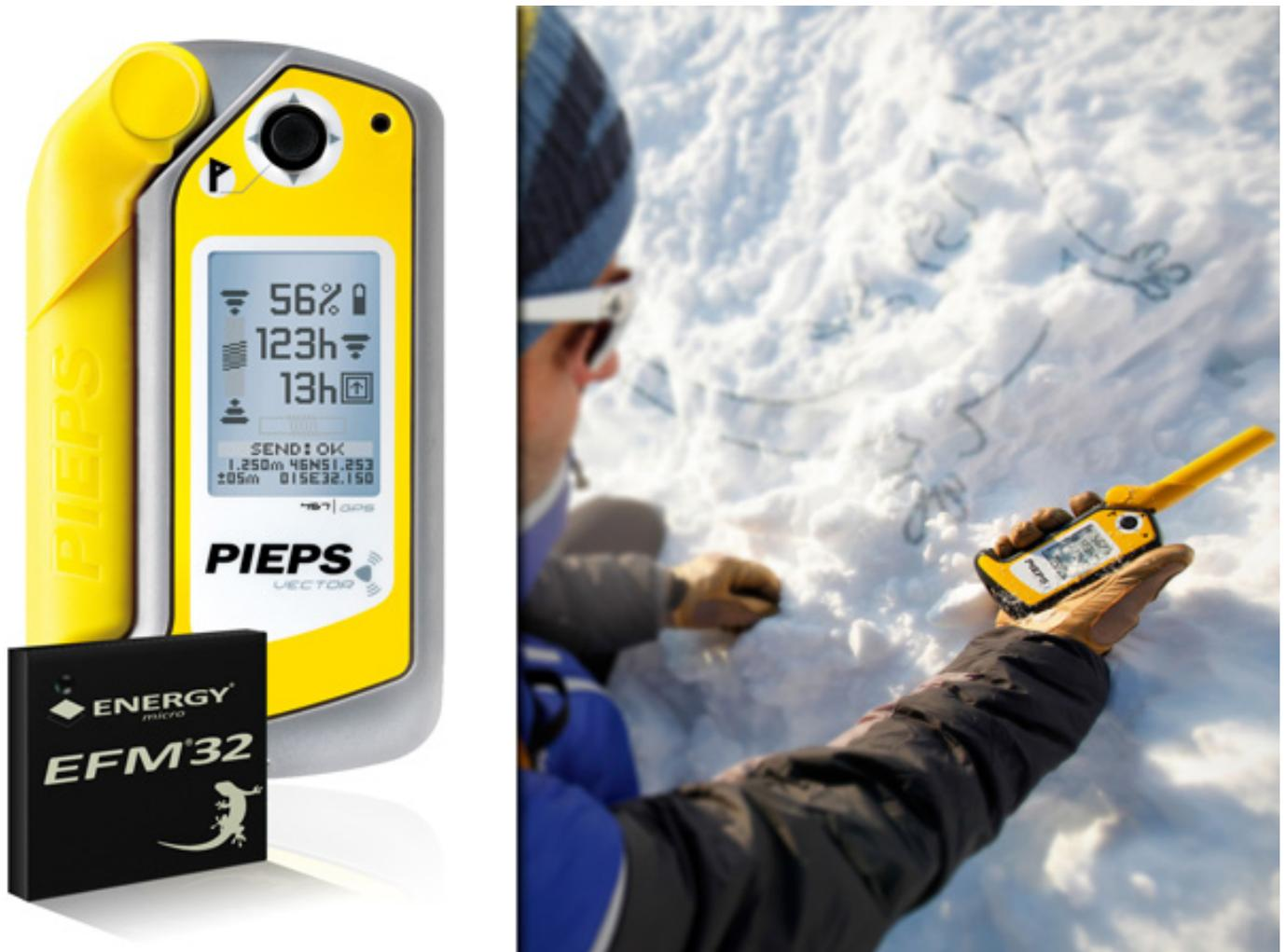
The new PIEPS VECTOR is the most advanced product of its type. The VECTOR introduces the possibility to record and display the user's location on a live map like a standard GPS and is a maintenance-free four-antenna beacon with rechargeable batteries. The device uses vector triangulation to pinpoint exact position and walking directions; the GPS-map displays and records exact co-ordinates for use either in emergency search or for later use on PC or laptop.
