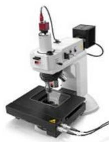
FRT MicroScope WLI is the new optical surface measuring system launched by Fries Research & Technology (FRT). Based on an optical microscope, it comes with a full white light interferometer for non-destructive measurement. This enables for quick and easy performing 3D measurements on a surface with very high vertical resolution. Especially it is a highlight for R & D departments and universities.
