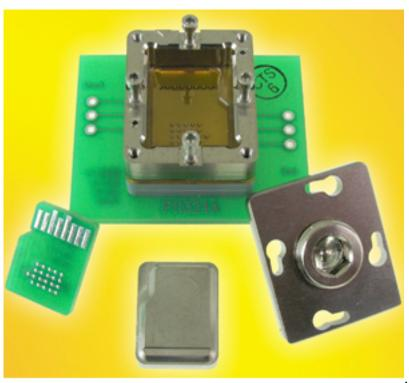
Ironwood Electronics recently introduced a new MicroSD socket (SBT-MicroSD-01) addressing high performance requirements for Speed Class Rating, which guarantees a minimum rate at which data can be written to the card. The contactor is a stamped spring pin with 19 gram actuation force per pin and cycle life of 500,000 insertions. Low force eliminates pin sticking issues due to temperature testing.
