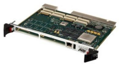
Extreme Engineering Solutions, Inc. (X-ES) introduces the XCalibur1600, a 6U CompactPCI Single Board Computer (SBC) supporting Freescale QorlQ P4080 processor. Available in either conduction-or air-cooled versions, the XCalibur1600 utilizes the eight Power Architecture e500mc cores running at up to 1.5 GHz, making it an ideal solution for high-end military, communications, and industrial applications.
