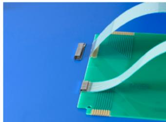
Molex recently released the ClipLok™ interconnect clip, an electomechanical connection that easily attaches to secure a membrane switch or FPC tail firmly to a printed circuit board, eliminating the need for mating connectors at each point. A first-to-market product, the low-profile ClipLok interconnect clip provides immediate and reliable circuit-to-board connectivity in a range of consumer, medical, networking and telecommunications applications.
