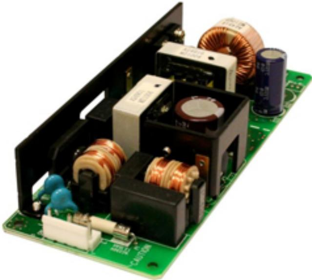
TDK-Lambda has unveiled its latest addition to its ZWS line of compact AC-DC pcb-mountable power supplies. The new single-output ZWS-BAF series are 100 and 150-watt supplies that accept a very wide AC input range, have a low profile of 1.3 to 1.45" and compact footprints of 2.44" x 6.1" or 3" x 6.3", making them an ideal choice for applications in light industrial, LED signage, test & measurement, gaming, point-of-sale and IT equipment.
