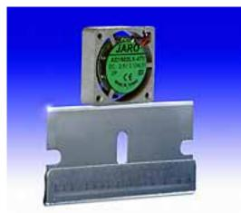
JaroThermal's "Super-Flow Micro" fan measures 15 mm  $\times$  15 mm  $\times$  4 mm while working at 26,000 rpm and producing .3 CFM of supercooled air. The low level of power consumption, which comes from a 2.5V DC operating voltage, makes the fan suitable for PDA, cell phone, hand-held test equipment, and portable power suppliers. It was designed to withstand drop testing of over 7000G's of force and provide a minimum 50,000 hours of product-life.
