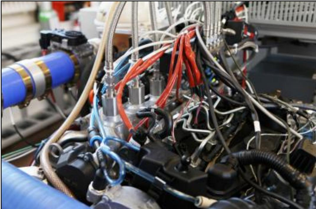
Researchers at ETH Zurich have developed an internal combustion engine that emits less than half the CO<sub>2</sub> compared to a regular engine without compromising performance. This corresponds to fuel consumption of less than 2.4l per 100km. This natural gas-diesel hybrid engine is based on a system of sophisticated control engineering.
