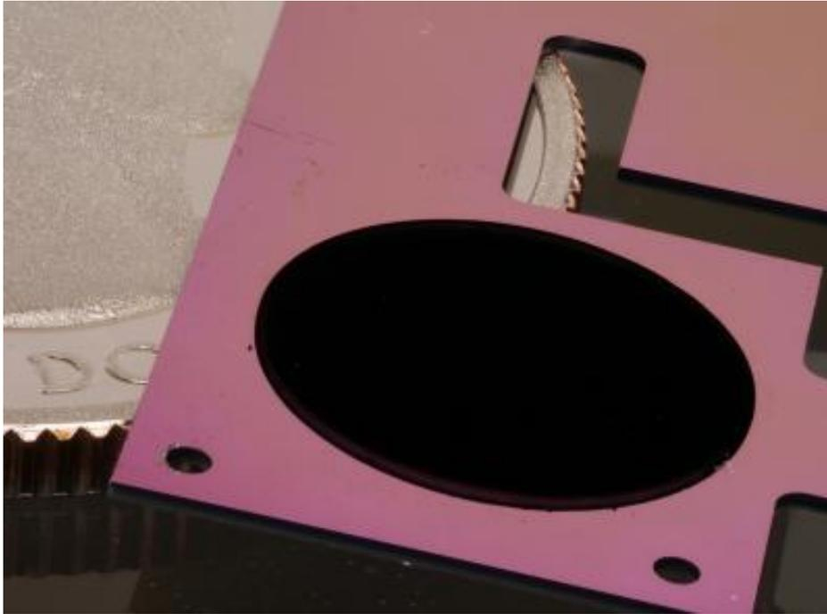
The National Institute of Standards and Technology (NIST) has demonstrated a novel chip-scale instrument made of carbon nanotubes that may simplify absolute measurements of laser power, especially the light signals transmitted by optical fibers in telecommunications networks.
