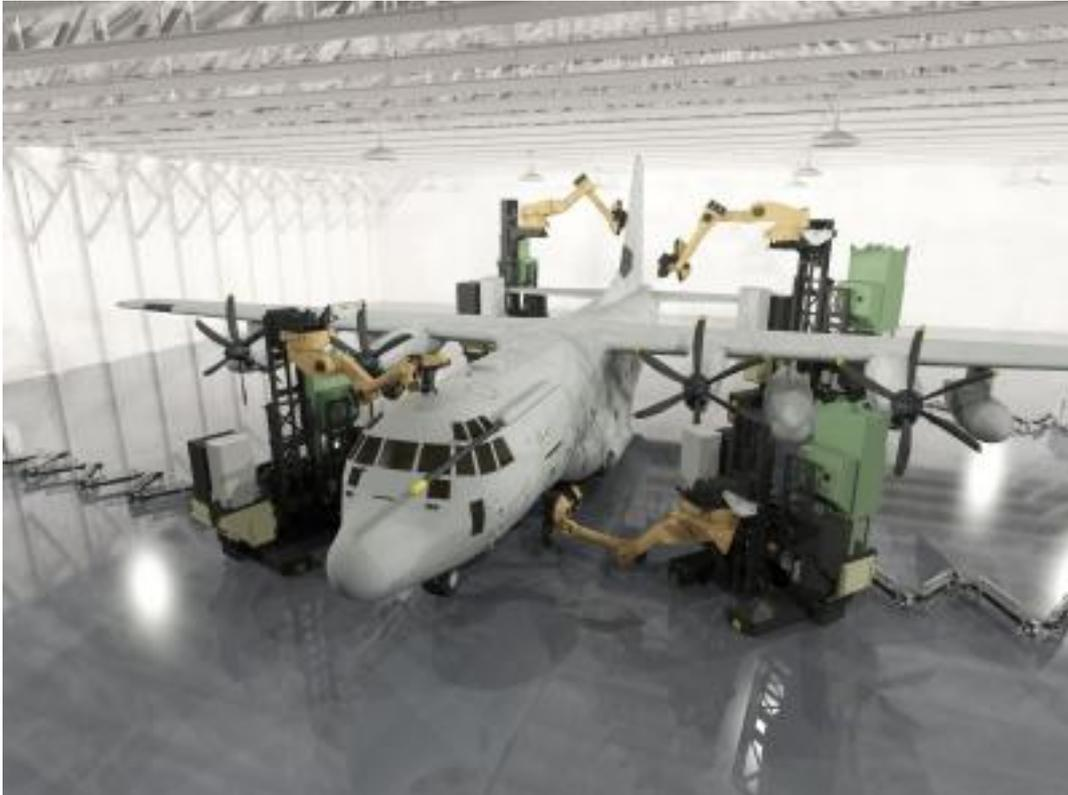
PITTSBURGH—Carnegie Mellon University's National Robotics Engineering Center (NREC) and Concurrent Technologies Corporation (CTC) of Johnstown, Pa., are working with the Air Force Research Laboratory and Ogden Air Logistics Center 309 AMXG to develop and demonstrate a robotic system that uses high-powered lasers to remove coatings from fighter and cargo aircraft.
