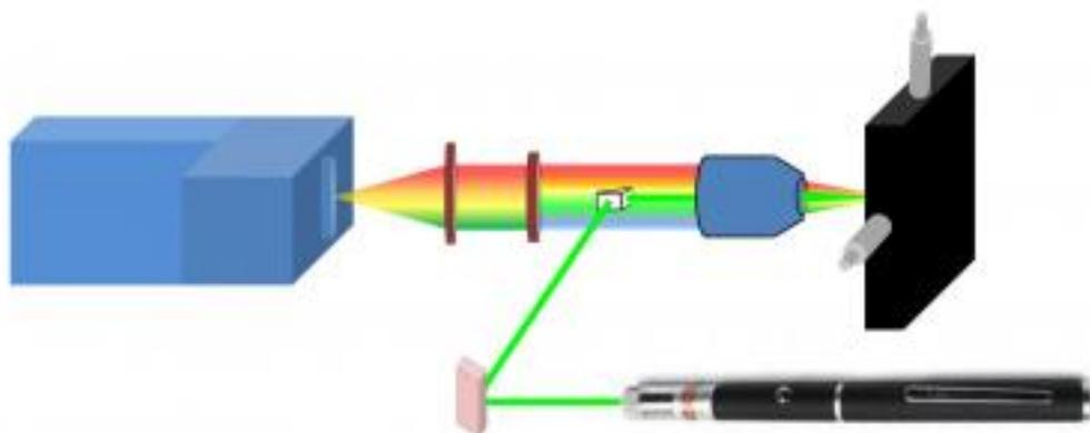
This is a schematic drawing of a Raman spectrometer, including a laser pointer, dichroic mirror, prism, objective, x,y translational stage, long wavelength edge filter, lens and a detector (spectrometer/intensified camera) coupled to the detector.
