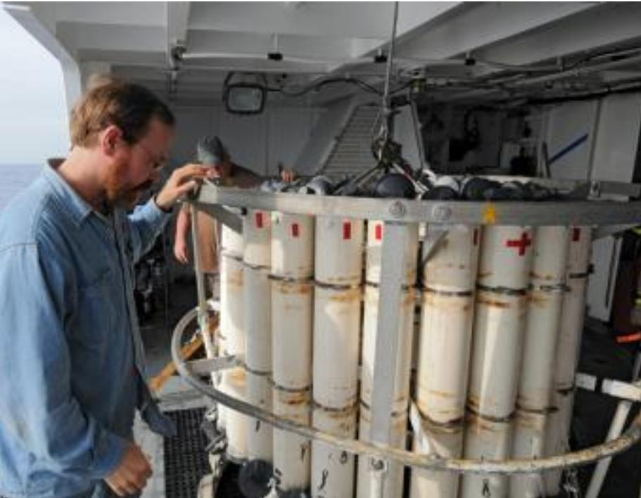
*WHOI senior scientist and marine chemist Ken Buesseler (foreground) checks a CTD sampler prior to deploying the instrument to collect data and water samples from the ocean off the coast of Fukushima, Japan.*
