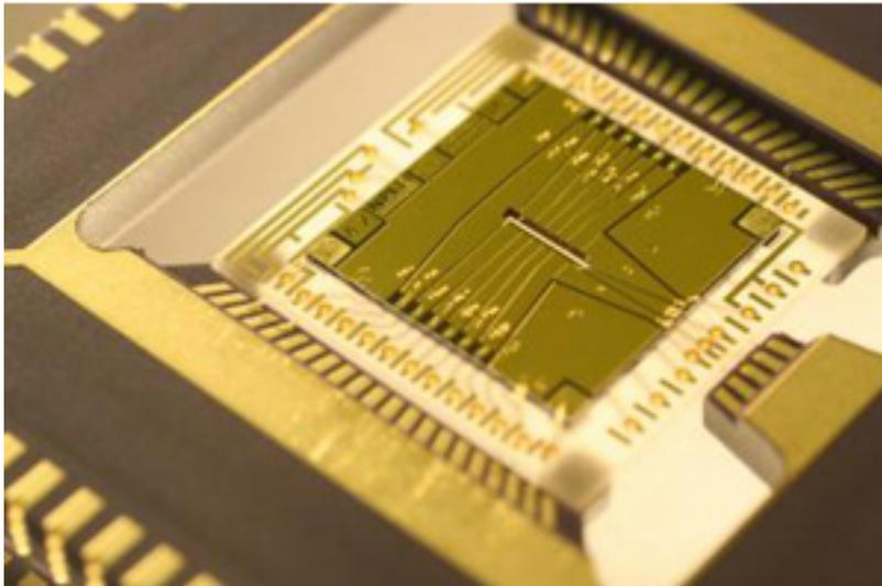
*Semi-conductor chip used by scientists at the National Physical Laboratory to test the first scalable 3D ion microtrap.*
