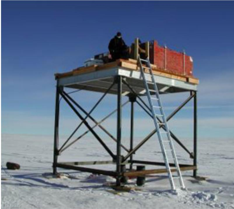
*This is the University of Delaware's "outside" neutron monitor at the South Pole. UD currently operates nine neutron monitors -- three in Antarctica (one inside and one outside South Pole Station, and one at McMurdo Station) and six in northern climes. The first neutron monitor installed at the South Pole has been in operation almost continuously since 1964.*
