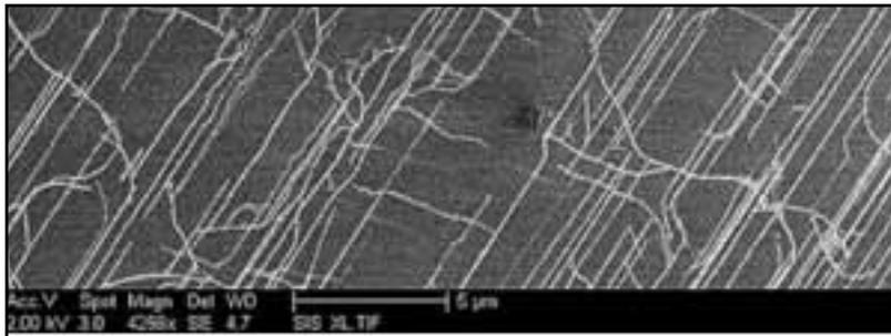
*Engineers from Stanford and the University of Southern California have found a way to design circuits containing carbon nanotubes that should work even when many of the nanotubes are twisted or misaligned.*
