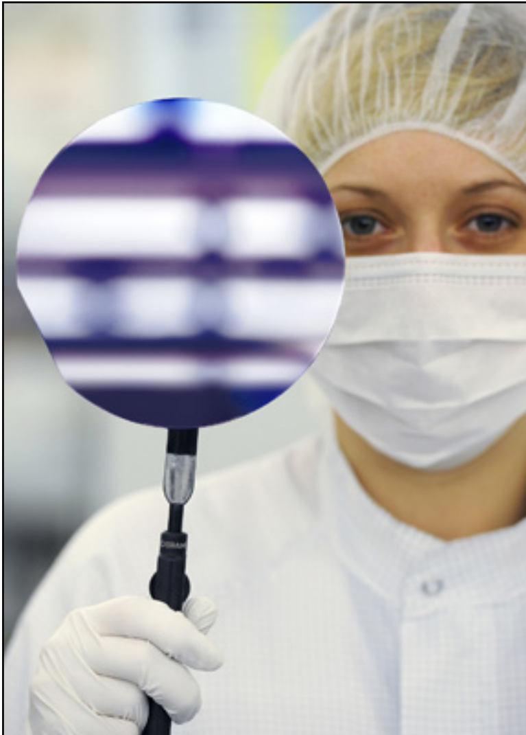
OSRAM high-performance LED chips based on InGaN technology today are fabricated on wafers with a diameter of 6 inches. Photo: OSRAM
