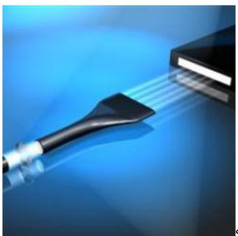
SCHOTT has developed a solution for forming "square" laser diode light into a homogeneous beam of light of any desired shape. The beam shaper is made of flexible glass fibers and can be coupled directly with the laser diodes. Collimation lenses are no longer necessary.
