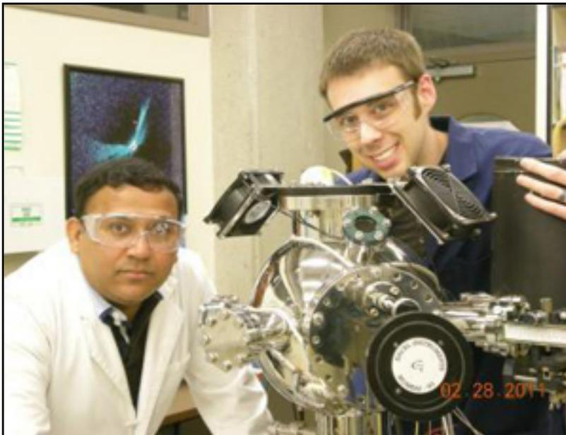
**University of Utah materials engineer Ashutosh Tiwari and doctoral student Nathan Gray have developed a way to align the magnetic "spins" of electrons within a silicon semiconductor chip at room temperature. The feat is a step toward faster, more energy efficient computers, phones and other "spintronic" devices that store data using the spin of electrons as well as their electrical charge.**
