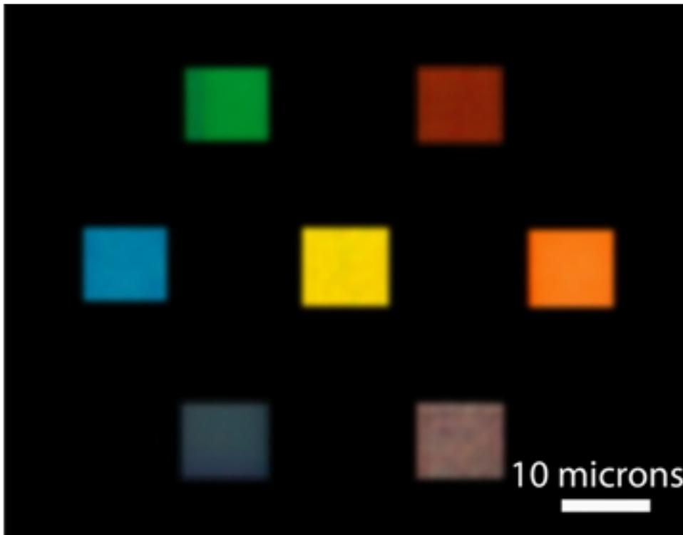
Because these new displays contain fewer layers, they would be simpler to manufacture, Guo said. The new color filters contain just three layers: two metal sheets sandwiching a dielectric. Red, green and blue pixel components could be made in one step by cutting arrays of slits in the stack. This structure is also more robust and can endure higher- powered light.
