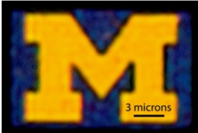
([University of Michigan](#) [1]) - In a step toward more efficient, smaller and higher-definition display screens, a University of Michigan professor has developed a new type of color filter made of nano-thin sheets of metal with precisely spaced gratings.
