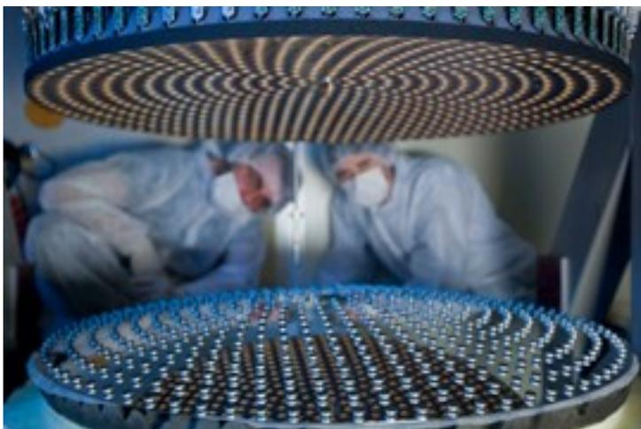
**Image one:** A picture of the movable secondary mirror during its installation in the Arcetri lab. The image shows the 672 tiny magnets spread over the back of the mirror. The reflecting face of the mirror is face down. The
