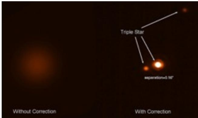
**Image two:** A double star as observed with the LBT in standard mode (left), and with the adaptive correction activated (right). Because of atmospheric blurring, the fainter companion of the star cannot be identified in the images taken in standard mode, while it is easily visible when the adaptive module is activated. A third faint star also becomes visible in the upper right part of the frame, thanks to the increased sensitivity of the telescope in adaptive mode.
