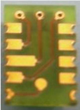
[1] Modules with [castellated mounting holes](#) [2] are showing up more and more these days. I've also heard it called a "half-via" setup. Both seem to fit. The copper mounting pads on the bottom of the module's little PCB wrap up the side of the PCB with a half-via. Thus, the name "half-via." If looked at from the base, the edge does look a bit like the outline of the top of a castle wall, so that makes sense too.
