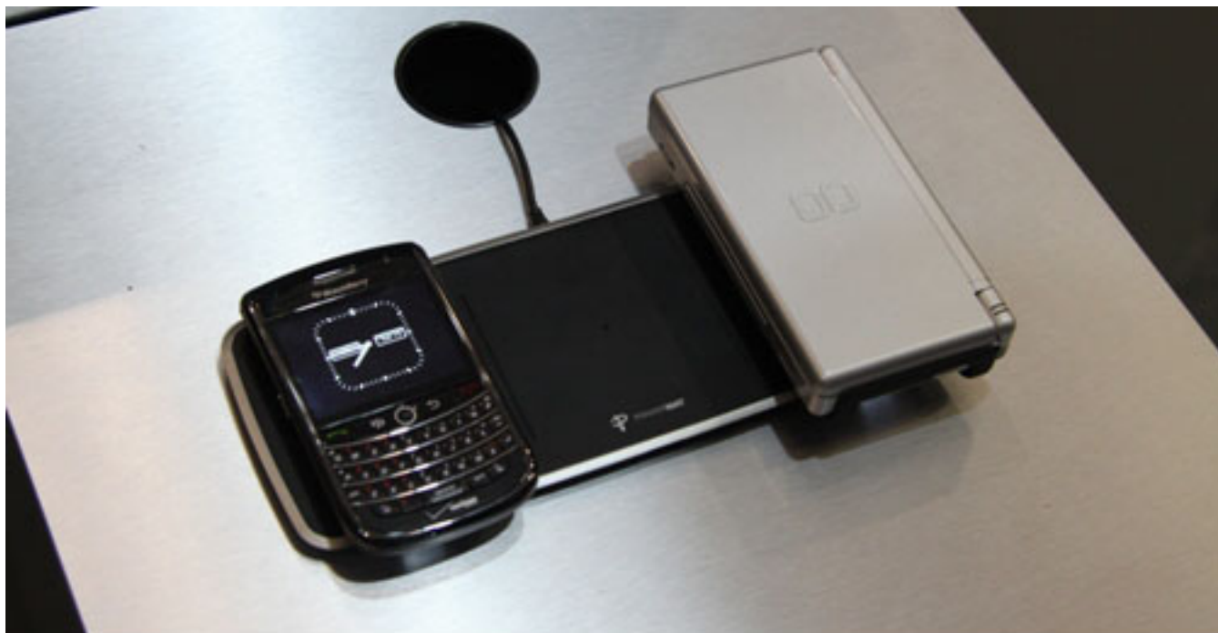
One of Powermat's device chargers (no cables required)--see video below.
