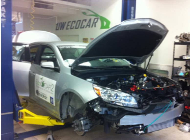
Another technical challenge has been the integration of our small diesel engine. The link between the Malibu's body control unit (BCU) and the new engine control unit (ECU) is a common wiring harness. The bulk of the wiring harness's connections are to engine sensors, so the new engine's harness is being used. Unfortunately, the new harness connector for the BCU is different than the Malibu's stock harness. Electrical sub-team lead Blake Simpson explains:
