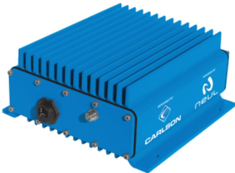
[3]The Neul and Carlson system will give users up to 16 Mbps of bandwidth for each available vacant TV channel and unmatched ability to make long range, non-line-of-sight links. Designed specifically for the needs of wireless Internet service providers (WISPs), RuralConnect has been priced to make it immediately commercially viable. Samples and development kits are available now, with volume shipments of the new system to start as soon as Q2, 2012.
