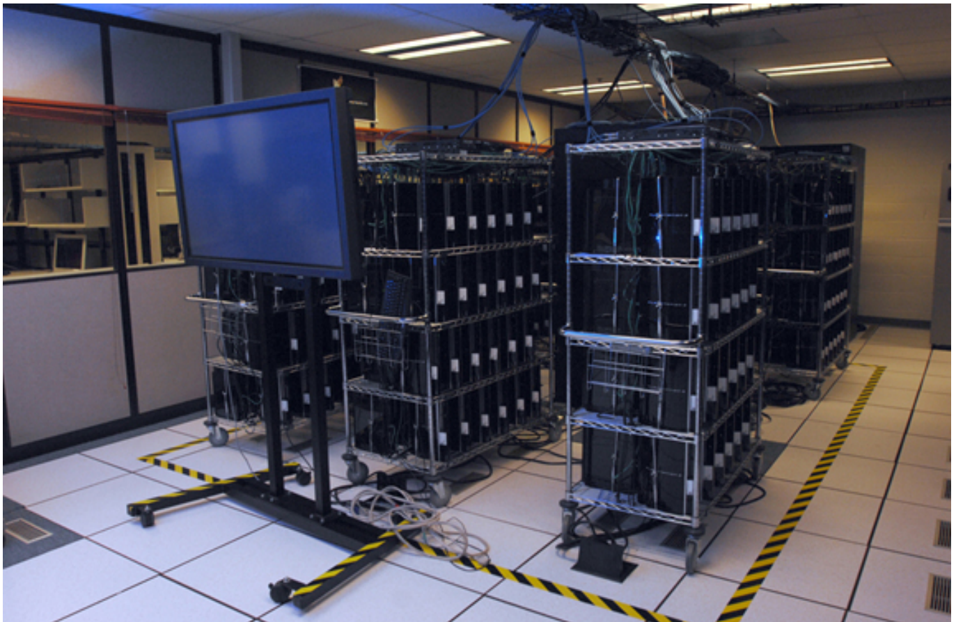
The original computing cluster using 336 PlayStation 3s.
