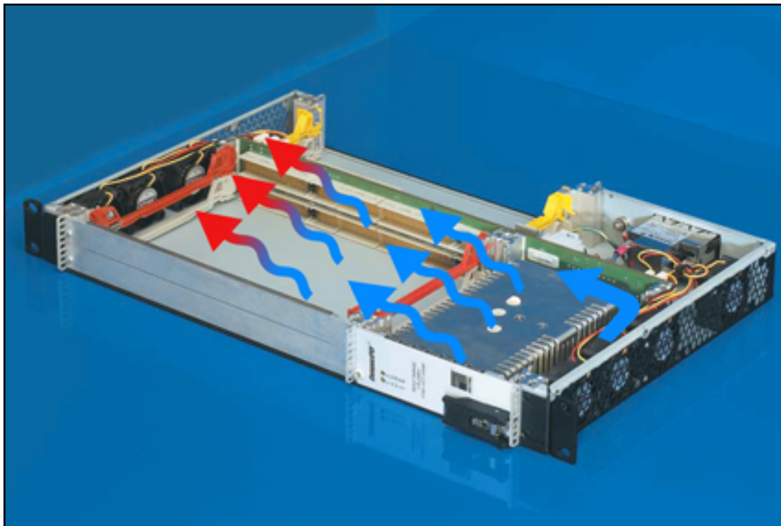
Figure 1. Side-to-side airflow path across a 1U Slimbox horizontal chassis.
