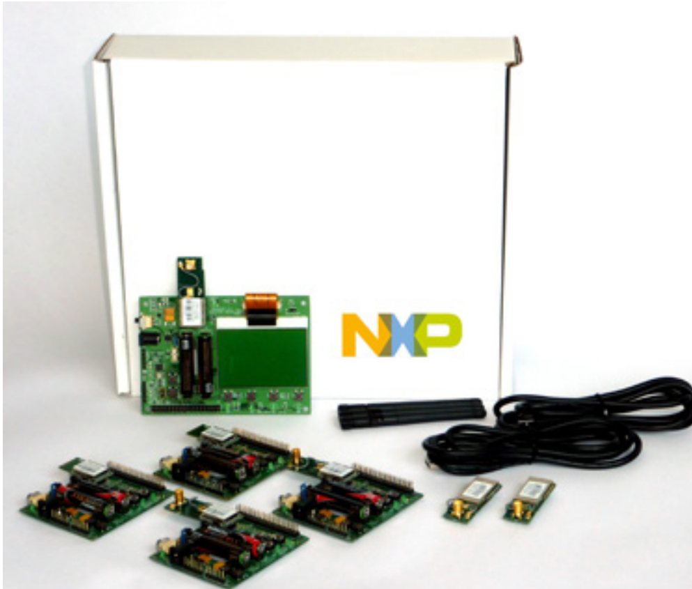
Figure 1. The JN5148 Evaluation Kit from NXP includes transceivers, software, and design tools help engineers get off to a quick start with a wireless sensor network.
