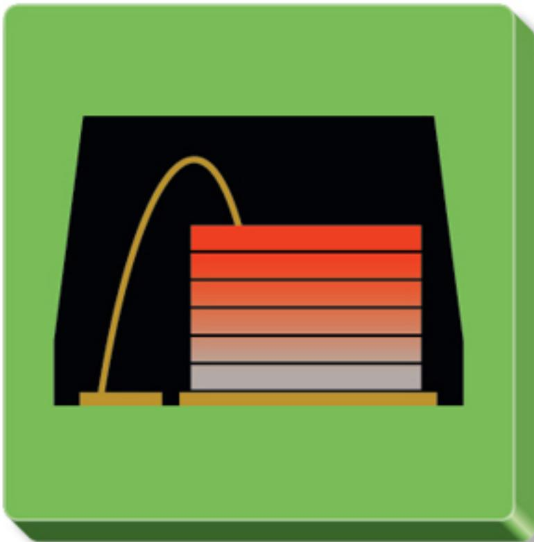
**Figure 2. Surface-mount TVS design with stacked die**
