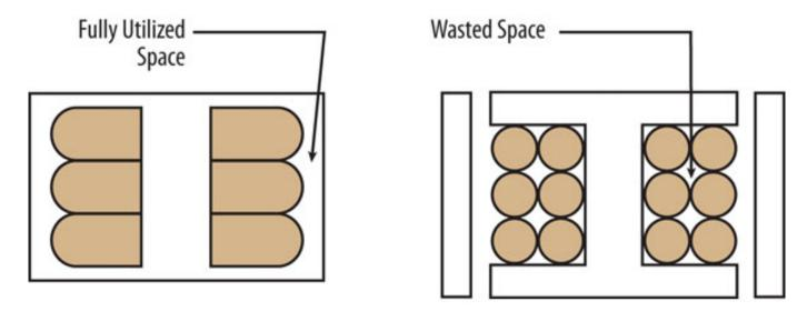
Figure 3. Powdered iron core makes the package efficient.
