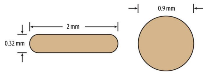
Figure 1. Cross-sectional area and surface area of flat and round conductors
