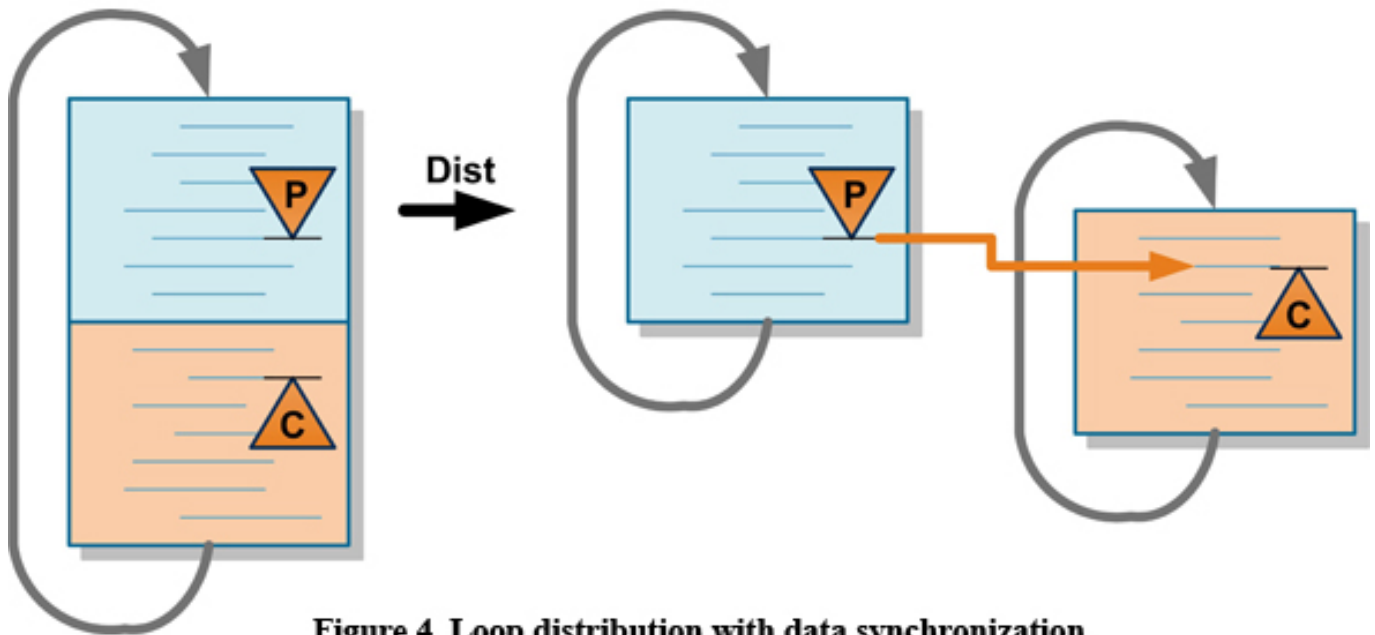
Figure 4. Loop distribution with data synchronization.
