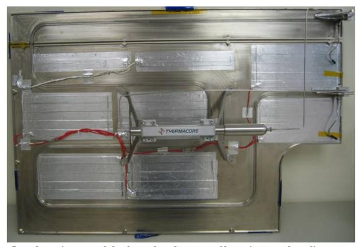
Loop heat pipes extend the thermal performance of heat pipes over long distances and give designers considerable flexibility in creating thermal solutions for satellite applications.
