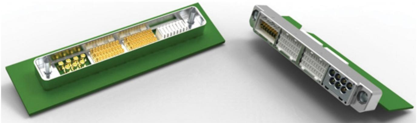
**Figure 5: Tyco Electronics High Speed Ruggedized Backplane Connector feature SMPM RF interconnects. Compliant pin motherboard and cable mount daughtercard modules shown.**
