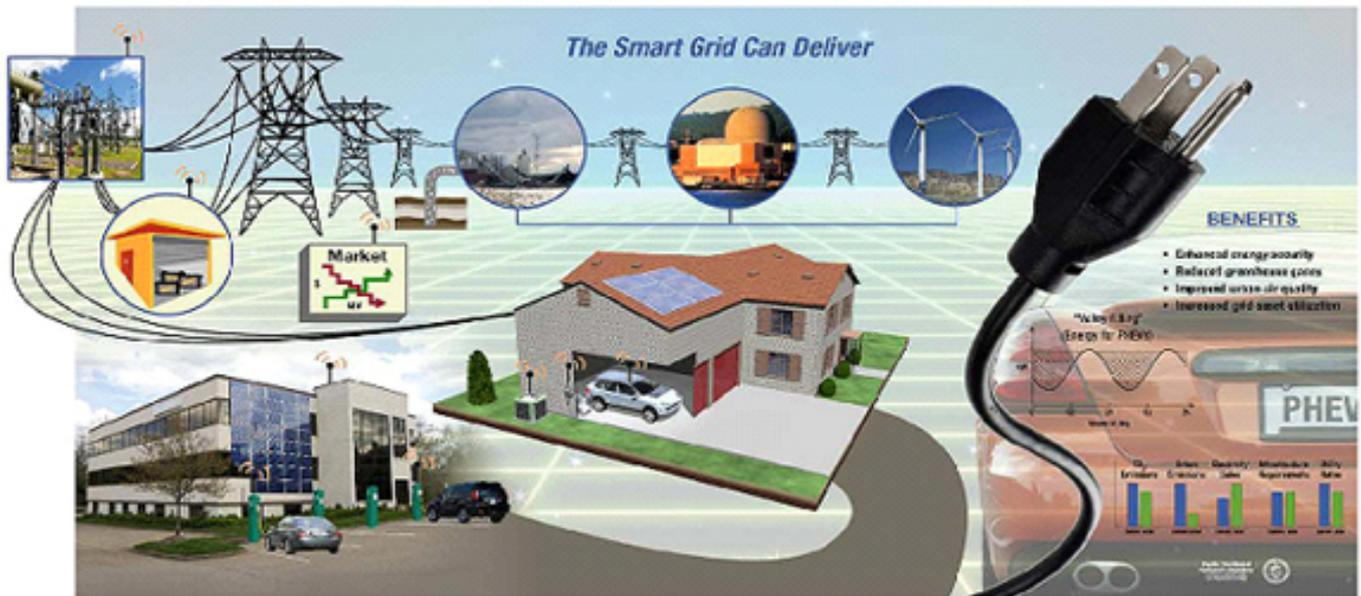
Distributed computing and communications technology will be incorporated to deliver real-time information and enable the near-instantaneous balance of supply and demand down to the device level. In short, the smart grid will deliver electricity from suppliers to consumers using digital technology to save energy, reduce cost, and increase reliability and transparency.
