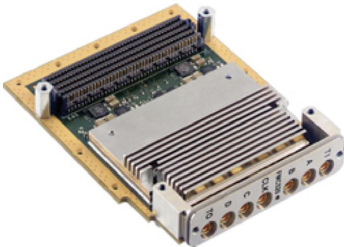
The FMC offers an elegant, simple solution because they only host I/O devices, such as ADCs, DACs or transceivers. FMC modules have no on-board processors or bus interfaces, such as PCI-X. Instead, FMC modules take advantage of the intrinsic I/O capability of FPGAs to separate the physical I/O functionality on the module from the FPGA board design of the module's host, while maintaining direct connectivity between the FPGA and the I/O interface.
