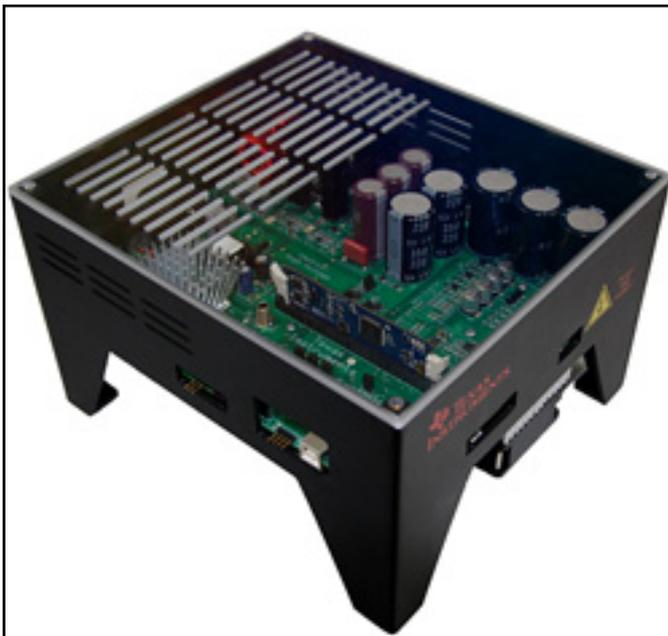
**Fig 1. The High Voltage PFC and Motor Control Developer's Kit from Texas Instruments includes a power factor correction stage under AC-induction, brushless-DC, and permanent-magnet synchronous motors.**
