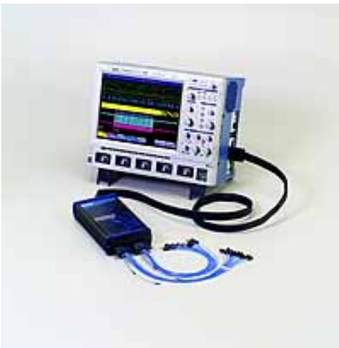
“When you plan to buy an analyzer or mixed-signal scope, ask how its probes will affect your signals,” cautioned Lauterbach. “You don’t want an instrument to corrupt your signals and cause additional problems, but engineers may forget about interactions between probes and the signals they want to explore. In general, you want any leads from your board to a mixed-signal scope to be as short as possible.”
