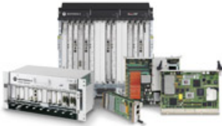
Figure. This collection of hardware shows an ATCA shelf populated with blades (background), two ATCA boards (right), a populated Micro TCA shelf (left), and a Micro TCA blade based on an AMC board (center). Courtesy of Motorola.
