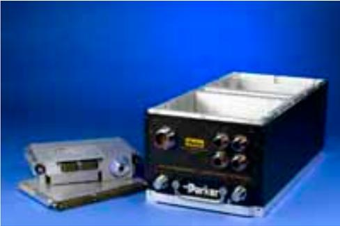
Parker-Hannifin concentrates its liquid-cooling technologies on commercial off-the-shelf (COTS) computer boards used in commercial, military and aerospace applications. The company's electronics enclosures with liquid-cooled side walls provide heat removal for conduction-cooled board modules that use a thermally conductive frame. Heat
